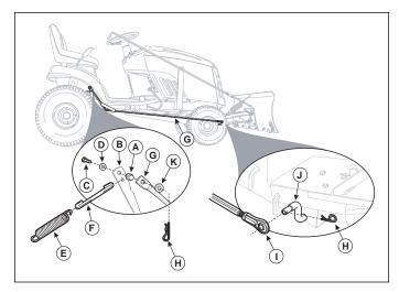
Figure 10. Belt Tension Lever
